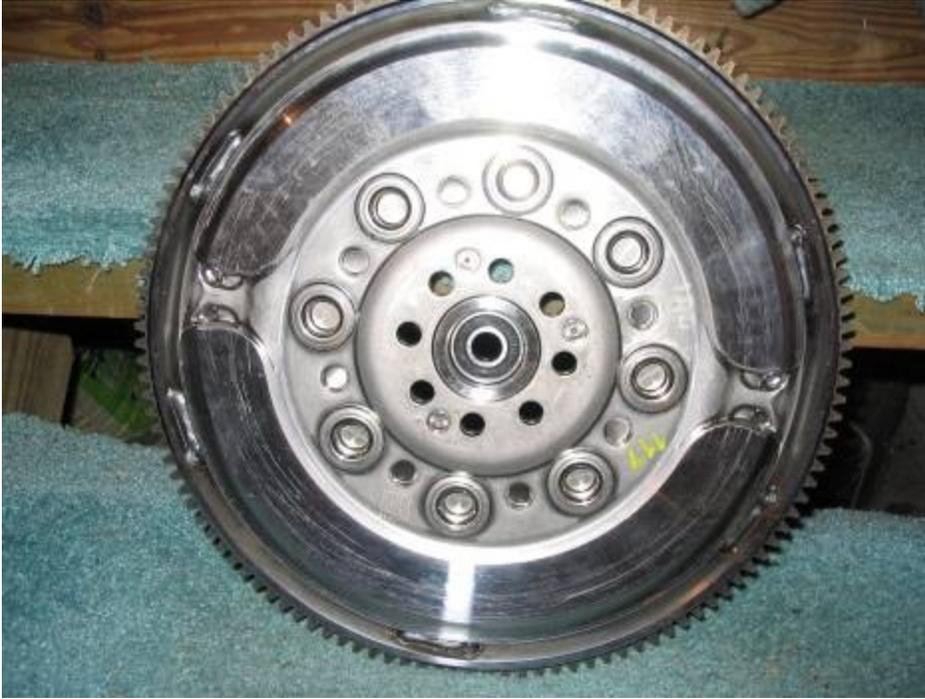
Back side of flywheel. The pulled side of the rivet is hidden by the small caps. In the picture above note that a few rivets and caps have been punched out (on the bottom).
