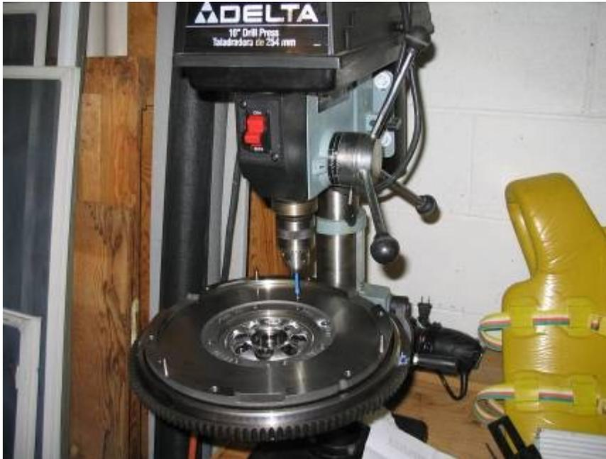
I used a drill press to ensure that the holes to be drilled were as dead-on as possible.
