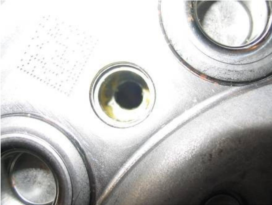
This is what the back side looks like where the rivet was punched through. You will note there is grease therein. This area houses the flywheel's greased planetary gears. Ideally some means to plug any gap after completing the flywheel installation should be included to keep debris out (to be determined).
