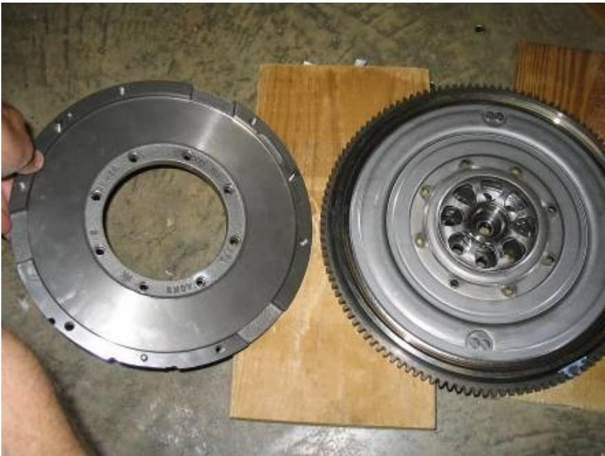
When you punch the last rivet the friction place will probably jar loose too. This picture shows it now removed (holding it). The flywheel holes are now ready to be tapped.
