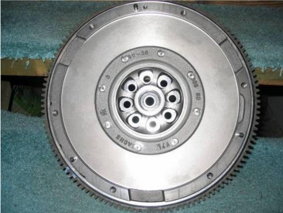
This is the dual mass flywheel (Subaru 12345AA010), front side, showing friction plate to be removed by drilling and punching out the 8 rivets in the area with writings/markings. The rivets each have an indentation where the rivet shank was pulled.
