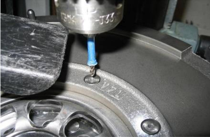
Using the existing rivet dimple I drilled first with a 1/8 in bit, no more than 15/32 inch deep. I marked this depth on the bit using tape. The black thing on the left is my vacuum nozzle. The picture above shows the 1/8 inch now drilled. The tape was bugged a little bit from shavings working their way up the bit.
