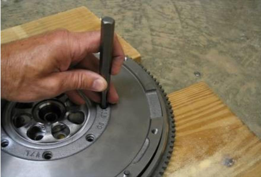
Place the flywheel on two boards such that the rivet can escape the back side when punched out. This was performed using a  $\frac{1}{4}$  in pin punch (which I happened to purchase at Home Depot – Lowes didn't have it at my store). The picture above shows all other holes with the rivets already removed. Center the punch and use a solid/heavy hammer, keeping the punch as straight as possible. The rivet should punch out with just a few light to medium blows.
