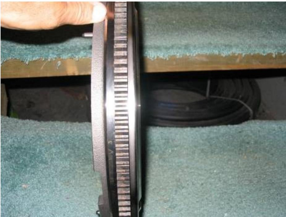
The flywheel profile. The side with the pins is the front side (this is the friction plate – my hand is on it).
