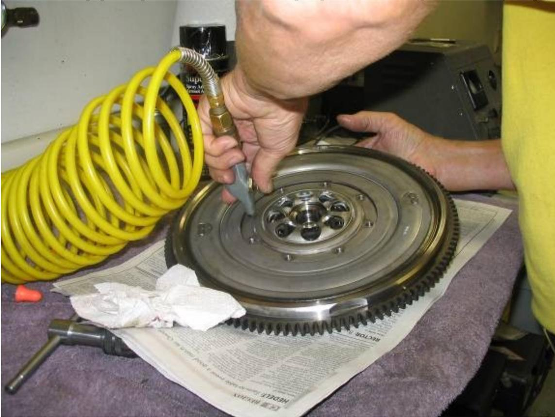
Now the flywheel should be ready to mount on the engine, once all other engine/plate preparations are performed.
