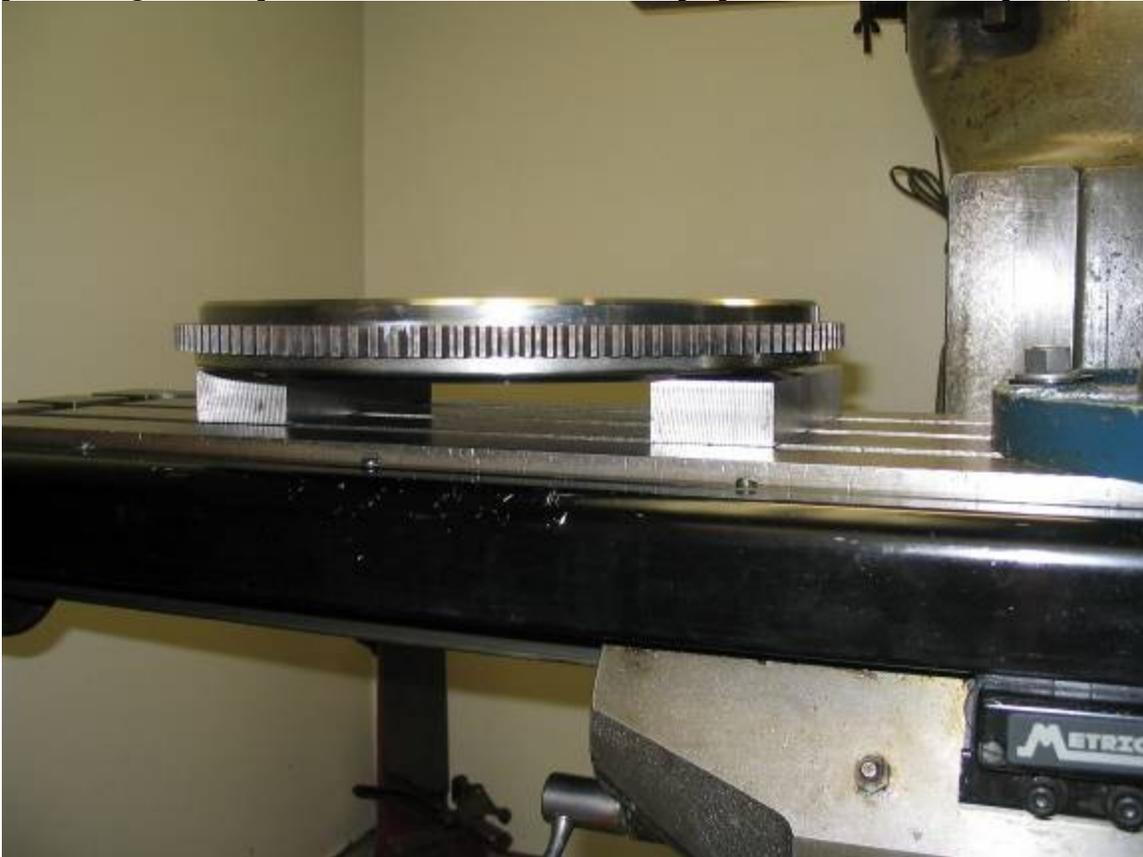
Next, in the picture below, the flywheel was clamped down. The point being that in your setup that you use some sort of clamp to keep the flywheel from moving while the tapping is performed.
