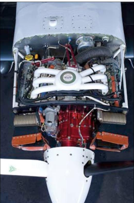
The H6 Subaru engine—a sophisticated double-overhead-cam six-cylinder design—is a tight fit in the RV-7 cowl. But it does fit!
