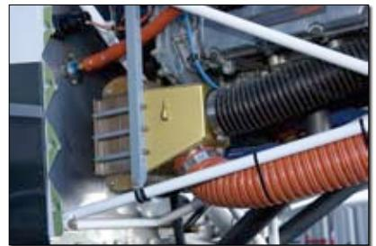
Simpson's "homebrew" oil-cooler arrangement uses 3-inch ducts taken off the forward air intake.
