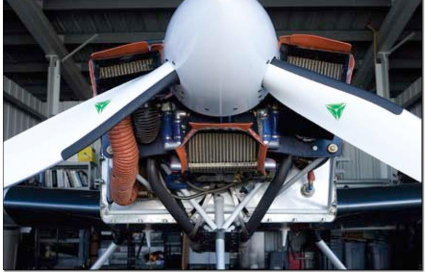
The modified water cooling system employs three small radiators around the prop; the current configuration has two larger radiators left and right of the PSRU.
