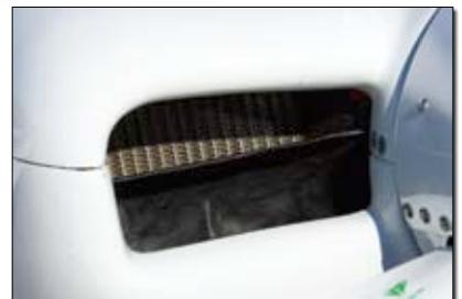
The horizontal duct borrows intake air from the copilot-side radiator and takes it back to the oil cooler. Precisely sizing and placing this splitter required many hours of trial-and-error testing.
