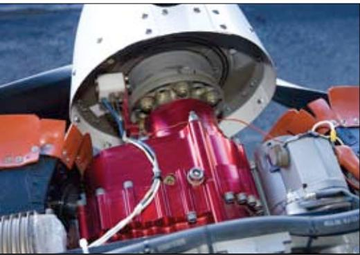
The Generation 3 PSRU, like its predecessors, is a two-shaft, four-gear arrangement meant to put the prop shaft on the same plane as the crankshaft.
